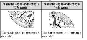
3. Turn the crown to adjust the setting if the leap second is not correct.
